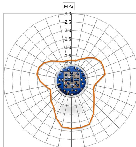
Figure 11: The total contact pressure profile over the shield
