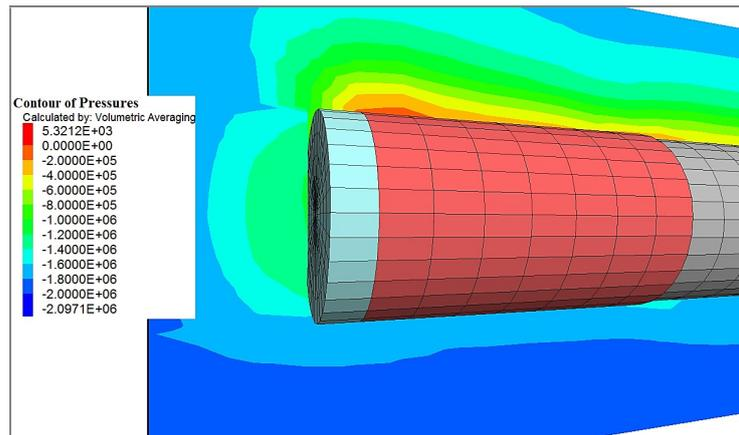
Figure 10: Contour of contact pressures around the shield
