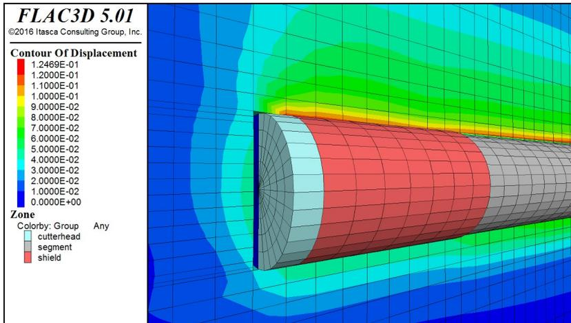
Figure 6: Contour of displacements around shield and segmental lining
