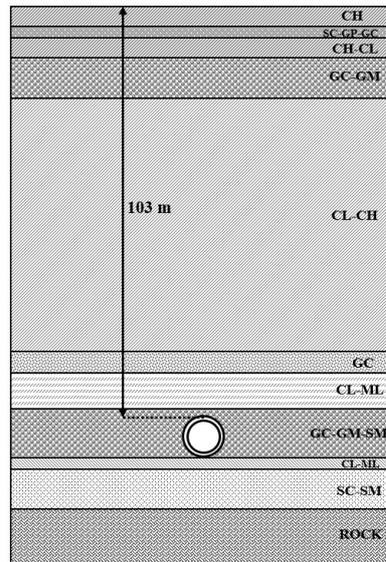
Figure 2: Geological cross section of the study area with tunnel location
