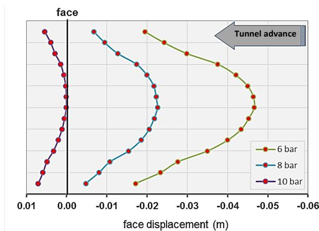
Figure 7: Displacement diagram at tunnel face resulted by applying different pressure values
