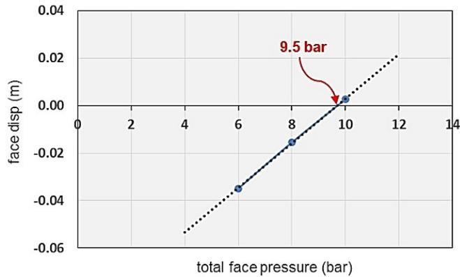
Figure 8: Displacement at tunnel face versus applied total face pressure
