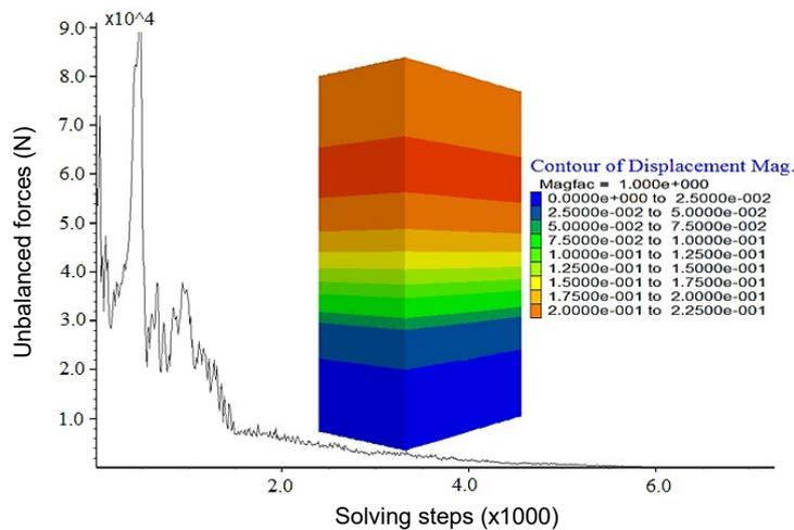
Figure 4: Contour lines of ground displacement after solving the block model for applying in situ pressures
