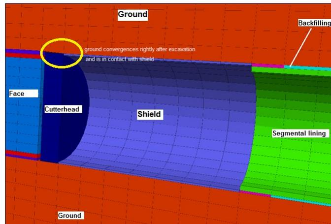
Figure 5: Screen shot of geometric configuration of the model of a EPBM in FLAC3D
