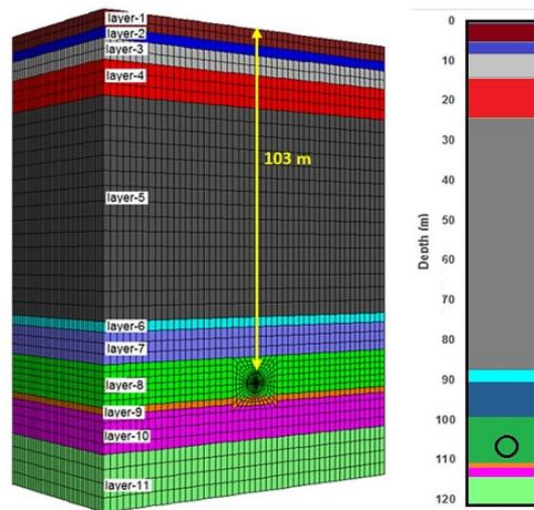
Figure 3: 3D model with the geological section of the study area
