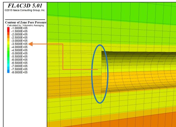
Figure 9: Contours of pore pressure (hydrostatic pressure) around tunnel face
